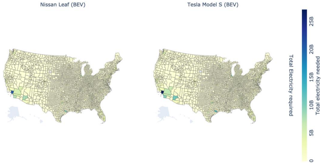
Figure S 9: Total electricity (in kWh) required to drive total NEI vehicle miles traveled for each electric vehicle.
