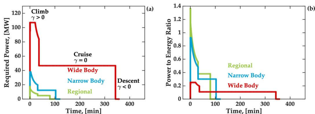
Figure 4. (a) Aircraft power profiles, along with conditions of flight in each segment. This figure illustrates the scaling challenges inherent in electric flight; as MTOM increases, the typical use case range also increases, causing a massive increase in the total energy needed. (b) Comparison of the power demand to energy (total energy over the trip) ratio throughout the mission.
