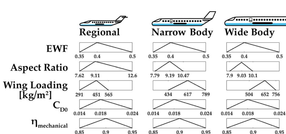
Figure 2. Parameters used to estimate specific energy for various classes of commercial aircraft. The minimum, maximum, and mean of each parameter and aircraft are shown on each plot. These parameters are used to estimate the power and energy of a prospective electric aircraft of each size. The data for these parameters are in the SI.
