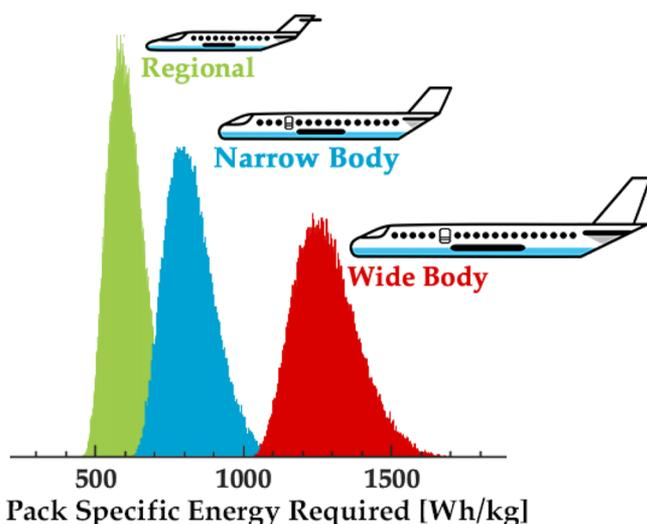
Figure 1. Histograms of specific energy for regional, narrow-body, and wide-body aircraft, illustrating the uncertainty stemming from aircraft design parameters. Larger (and longer-range) aircraft require a higher specific energy than do smaller (and shorter-range) aircraft.
